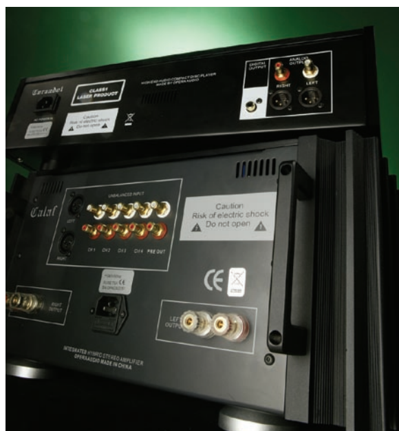
ABOVE: The rears of both units are uncluttered, the CD player sporting single-ended and balanced (XLR) outputs and the amp a single set of binding posts alongside four single-ended RCA inputs and one set of XLR balanced
